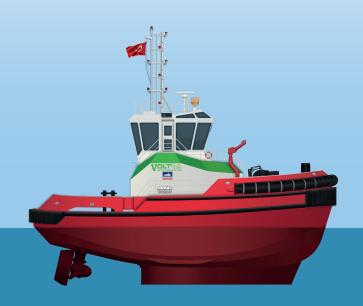
LENGTH OVERALL21.4 mBEAM, MOULDED11.3 mDEPTH, MOULDED4.0 mDRAFT, NAVIGATIONAL4.6 m
